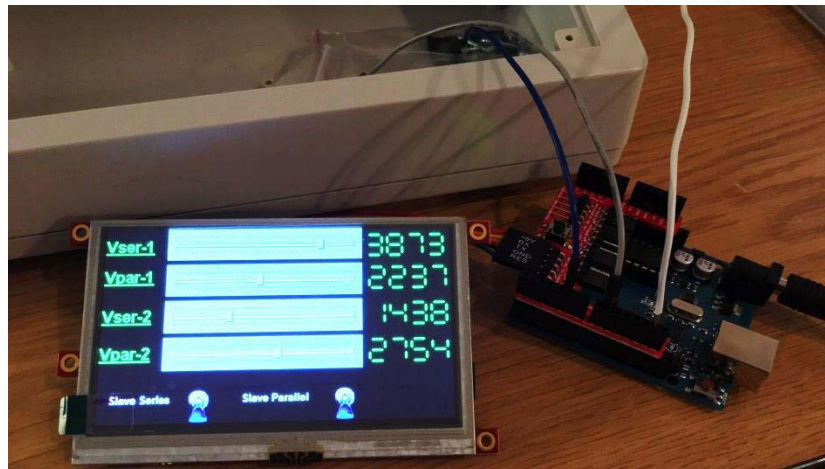
Figure 54 Arduino Uno with attached LCD panel for creation of varactor tuning voltages. Touch-sliders on the panel are used to individually adjust all four tuning voltages while the toggle switches make it possible to also slave the series and or parallel voltages to one another. The numerical display readout is in mV for each respective voltage.
