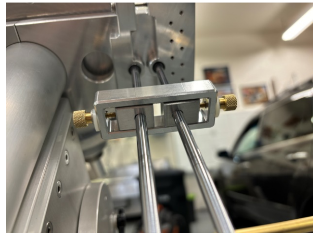
Figure 2 Original design which used a spanner below the main bearings to compensate for axle-bending and slight shifting of the (small) main bearings
