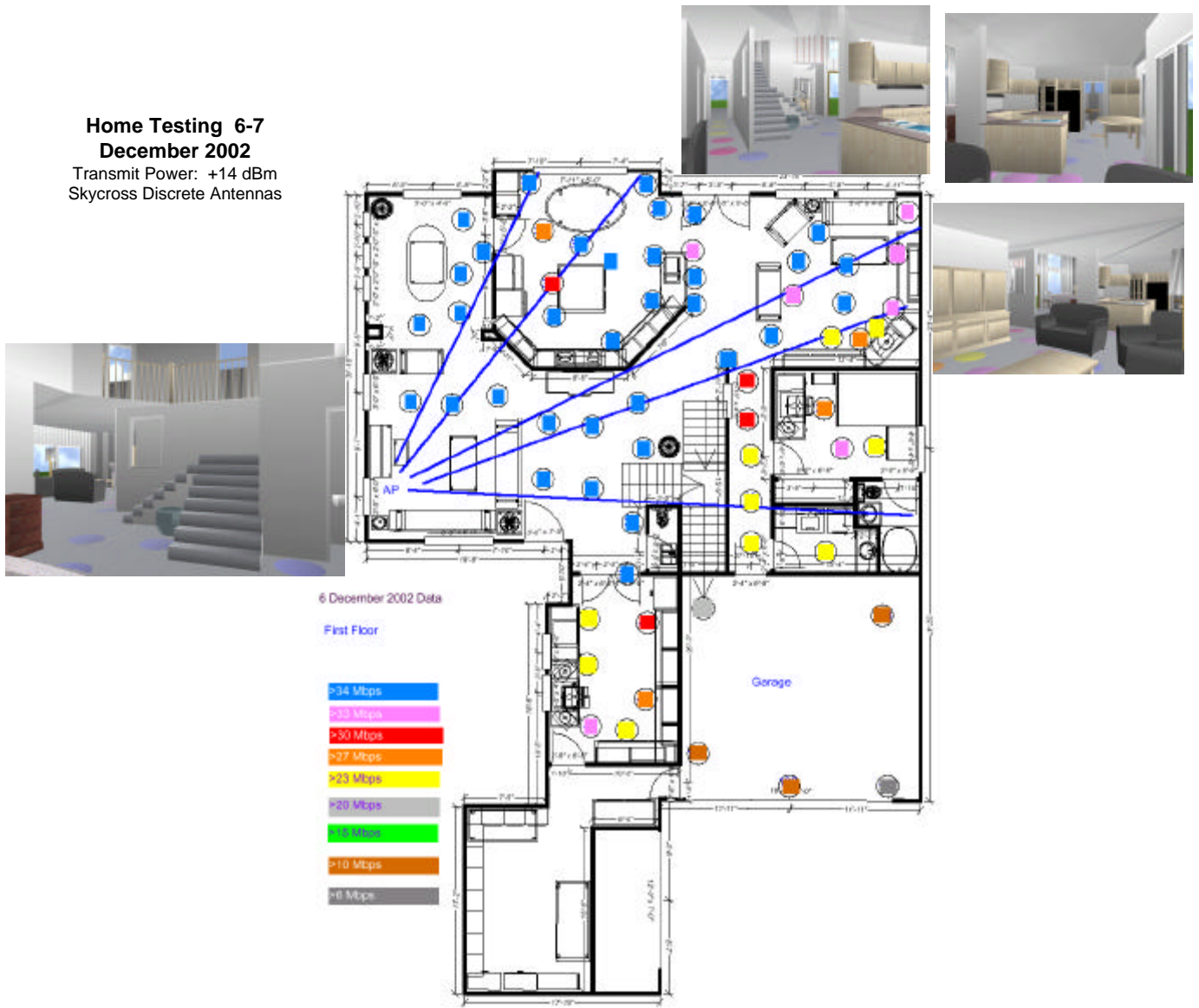
Figure 8 Data-Mode Collection Results for First-Floor (Maximum diagonal distance shown in main living area is approximately 60 feet.)
