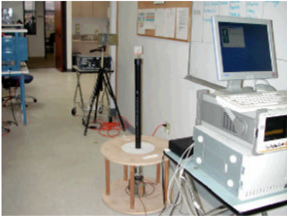
Figure 39 Portion of Antenna Gain Pattern Assessment Equipment Setup
