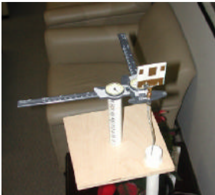
Figure 40 Simple Microstrip Patch Antenna Used to Examine Local 5 GHz Signal Energy. X- and Y-Axis Plastic Micrometers are Used to Accurately Position the Antenna for Each Measurement
