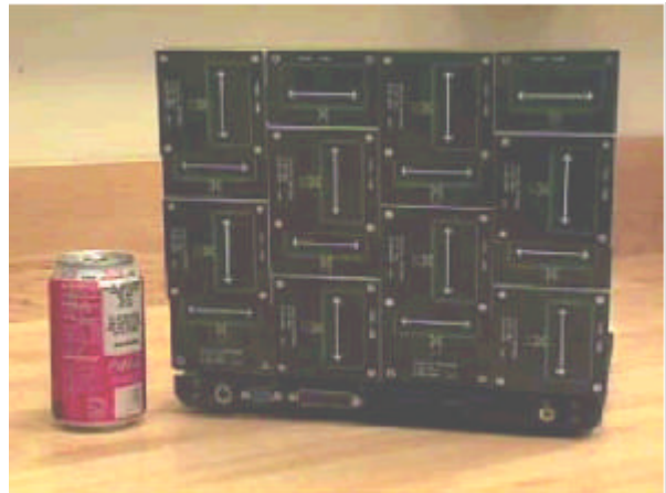
Figure 28 Multiple Antennas Integrated into Back of Laptop Computer (Lucent BLAST Technology) 9
