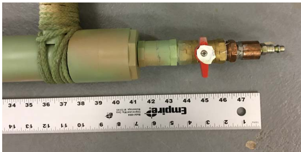
Figure 6 View of the air reservoir charging port. A standard 1" ball-valve was used with reduction down to the quick-connect which works with my workshop air compressor. Sweating the copper elements together was the only construction step which required special consideration.
