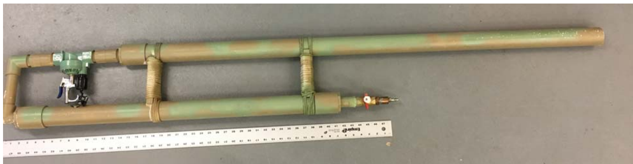
Figure 4 Spud cannon built primarily using 2" PVC. A 1" modified lawn sprinkler valve is used as the control valve between the pressurized air reservoir and the barrel. The ruler is 48" long.
