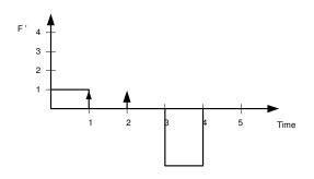
After taking the second derivative, we have only delta functions, and derivatives of delta functions as shown below.
