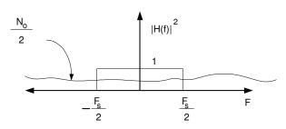
Assuming that the process is wide-sense stationary, the Weiner-Khinchine theorem can be used to compute the autocorrelation function as the Fourier transform of S(f) as
