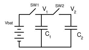
Close switch SW1, and capacitor  $C_1$  is charged to voltage  $V_1$ = Vbat. Now open switch SW1.
