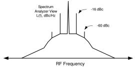
The most obvious question is that if the discrete spurious lines are phase-only, why are the second harmonic spurious terms so much lower in amplitude. If these are truly PM spurs, their levels are dictated by Bessel functions per traditional PM/FM theory, and it is not possible to have the further-out discrete spurious levels this low when the spur levels close-in are this high.
