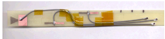
Figure 24 "Whip" Antenna Array Prototype Shown with Micro-Coax Connecting Each Antenna Element (Less Any Plastic/Rubber Sheathing). (Bow-Tie Element is at the Far Left.)
