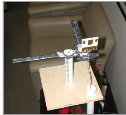
Figure 39: Simple Microstrip Patch Antenna Used to Examine Local 5 GHz Signal Energy. X- and Y-Axis Plastic Micrometers Are Used to Accurately Position the Antenna for Each Measurement
